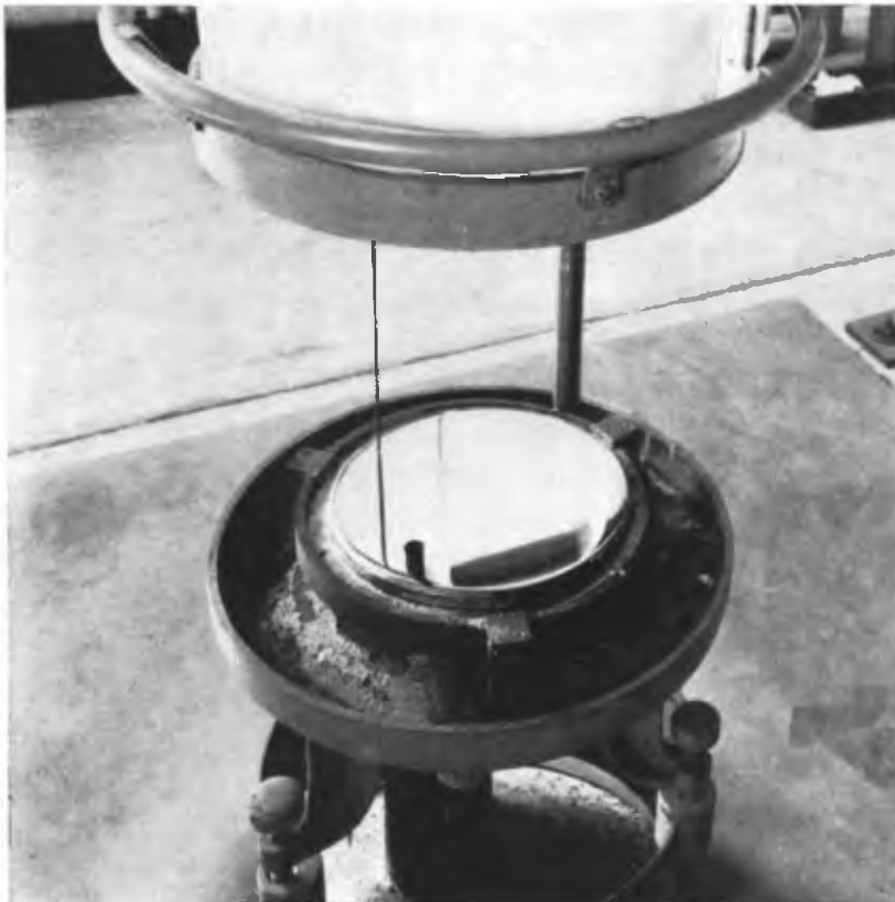
MERCURY MIRROR provides a flat and truly level surface. It is raised or lowered to focus the star image on the photographic plate under the lens. Above the surface of the mercury is a rod; its reflection can also be seen in the mercury. When the tip of this rod just touches the surface of the mercury, the image is in exact focus at the photographic plate.
