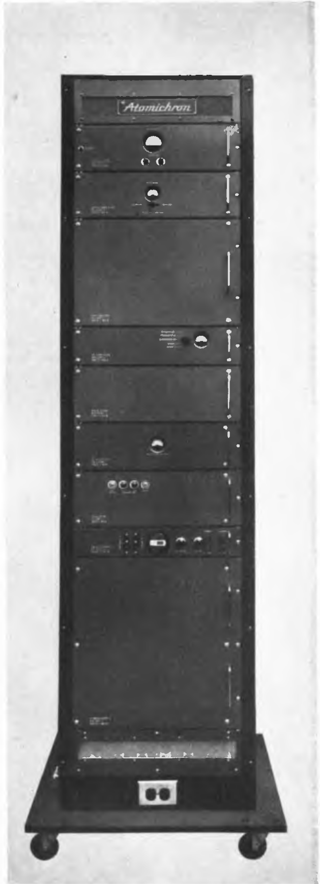
tube to target chamber at top. Deflecting magnets are behind the two rectangular plates. This device is made by the National Company. It is the first commercial atomically controlled oscillator.
